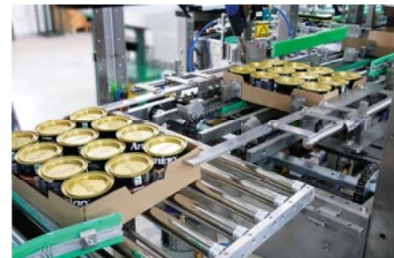
Direct connection to Shrink Wrapper
